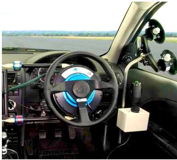
By combining the path-following technology with the Brake and Accelerator robots, it is now also possible to perform tests without a driver in the vehicle where the risk for the driver would be high or where the testing condition is arduous for the driver.
